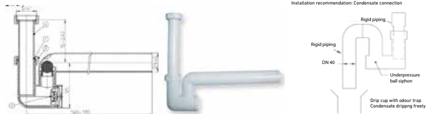
Fig. 1 Installation recommendation: Condensate connection
