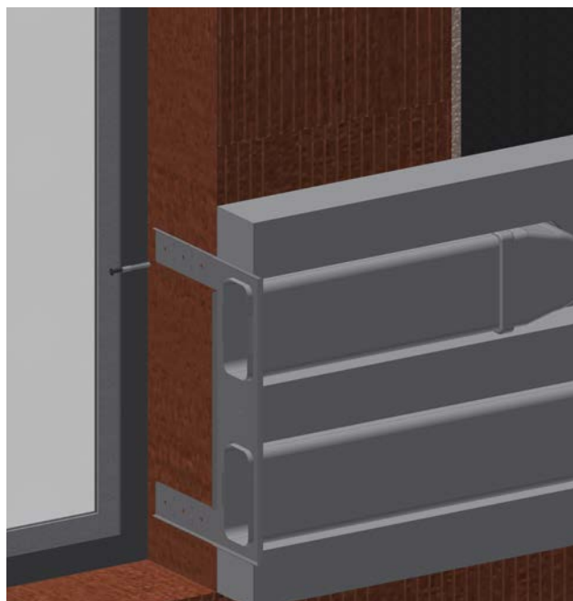
Fastening the mounting plate
