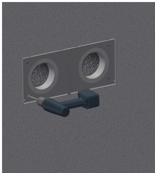
Use a 6 mm drill to pre-drill the EPP wall duct
