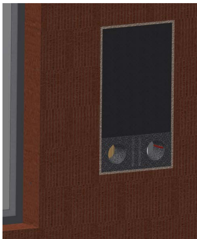
Wall duct flush with masonry
