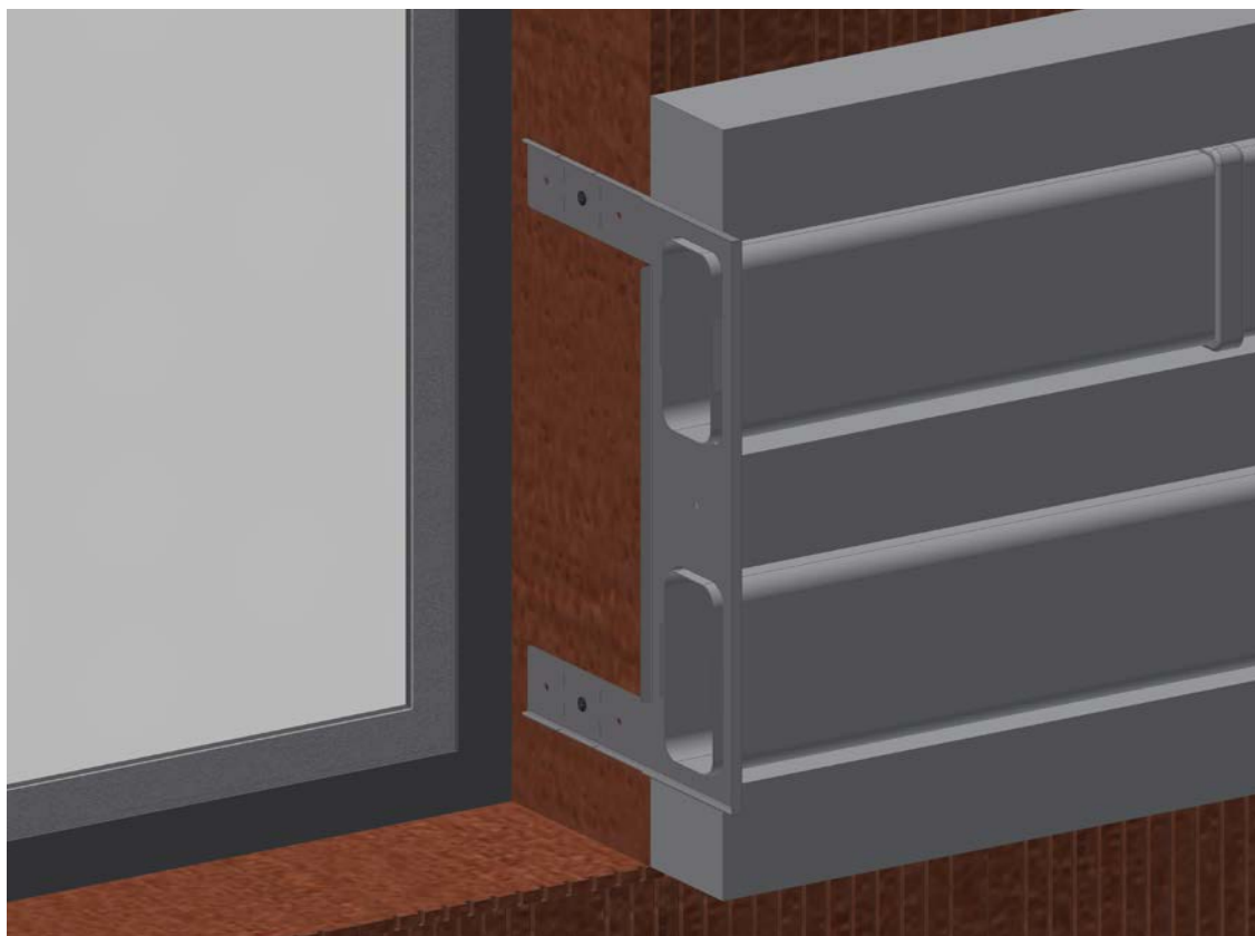
Installed mounting plate
